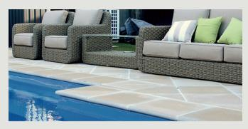
Bullnose pavers are a smooth, rounded edge as an alternative to the standard straight edge. Most commonly used on pool edges and steps.
