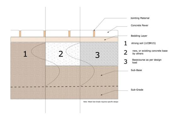
**Jointing Material** The jointing material can either be a sand or grout
