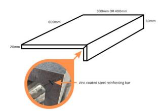
If cutting drop face pavers that have a zinc-coated steel rod, please ensure the exposed steel area is sealed with tile adhesive or a waterproofing agent.
