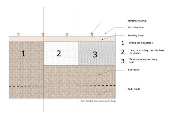
**Jointing Material** The jointing material is usually grout
